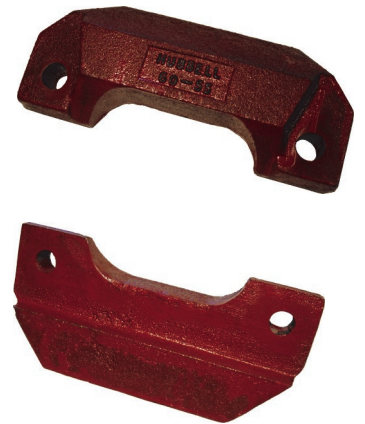
#60-55° Plow Shoe Ni -Hard Casting. To suit one-way plows, 8" hole centres.
